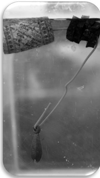
Figure 4: 10 gram weight floating with cork and pieces of neoprene
