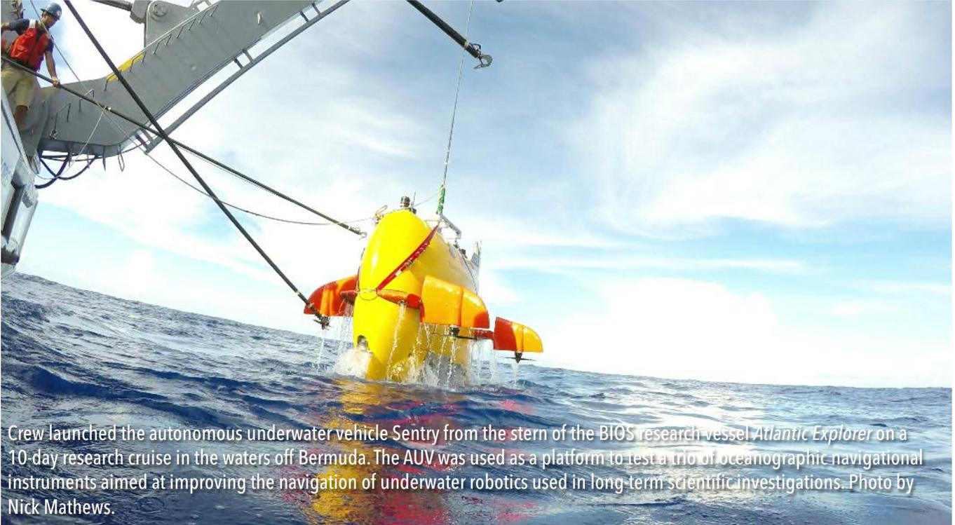
Crew launched the autonomous underwater vehicle Sentry from the stern of the BIOS research vessel *Atlantic Explorer* on a 10-day research cruise in the waters off Bermuda. The AUV was used as a platform to test a trio of oceanographic navigational instruments aimed at improving the navigation of underwater robotics used in long-term scientific investigations. Photo by Nick Mathews.
