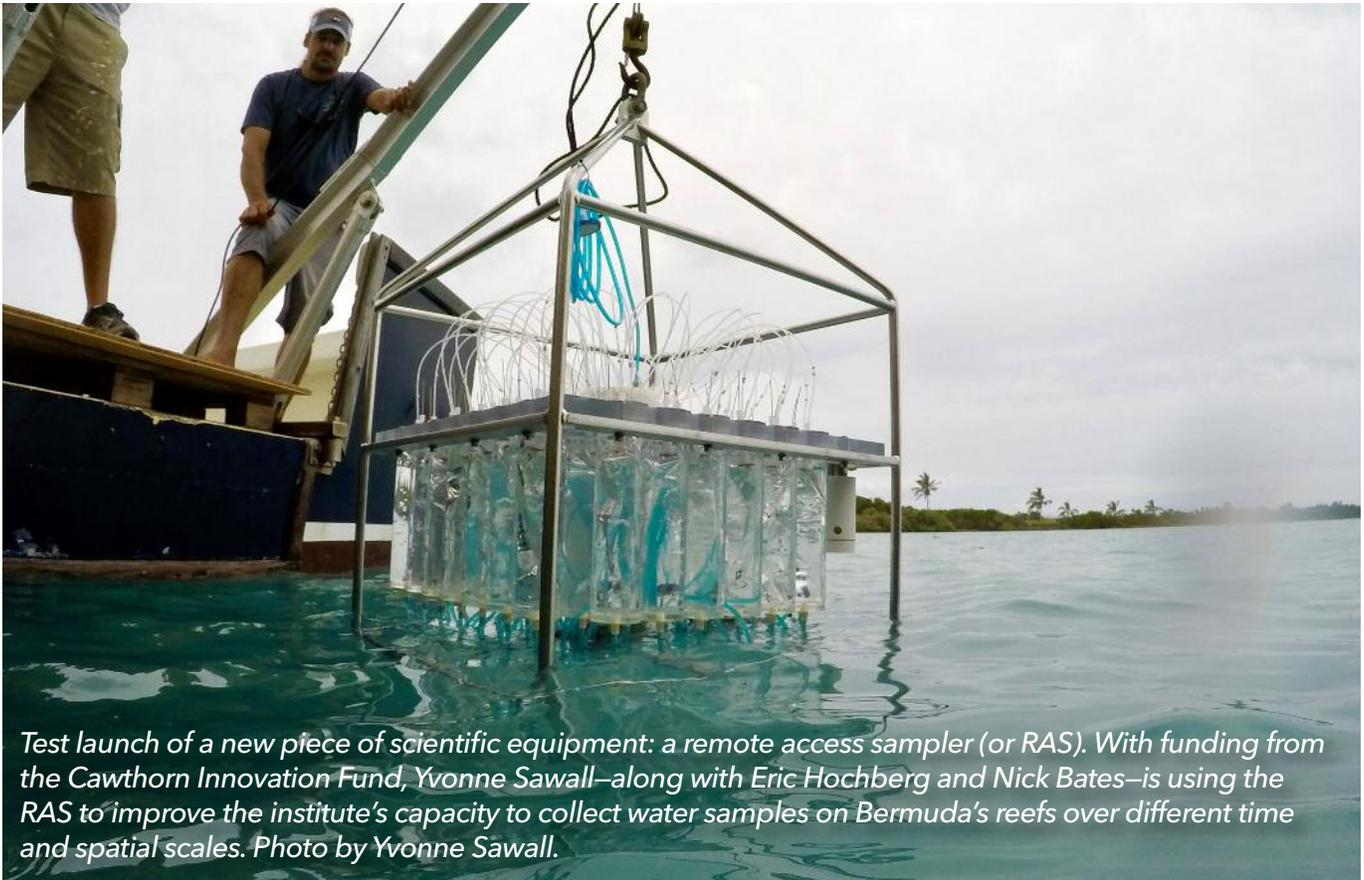
*Test launch of a new piece of scientific equipment: a remote access sampler (or RAS). With funding from the Cawthorn Innovation Fund, Yvonne Sawall—along with Eric Hochberg and Nick Bates—is using the RAS to improve the institute’s capacity to collect water samples on Bermuda’s reefs over different time and spatial scales. Photo by Yvonne Sawall.*
